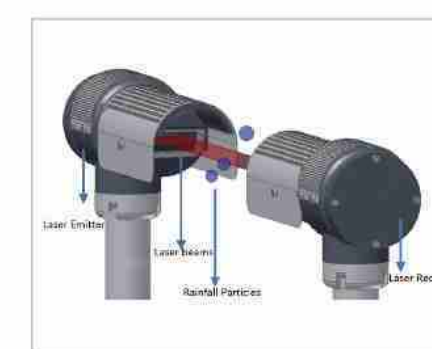
Disdrometer working principle
